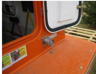
External water connection at right side below door
